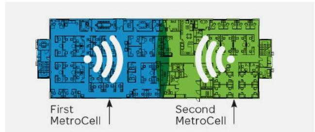
3. Find a site for the 2nd MetroCell that is as far away from the edge of the coverage area identified in step 2 as that edge is away from the first MetroCell. Map the coverage area as in step 2.
