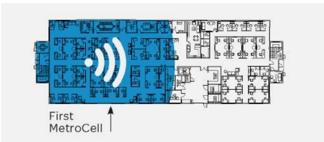
2. Map out the effective coverage area of the first MetroCell by walking around while looking at the number of “bars” of signal strength on a handset. Identify the edge of the area covered by the 1st MetroCell where signal strength is between 1 and 2 bars. This is as far away from the first MetroCell as a user could be and still be properly served by that MetroCell.
