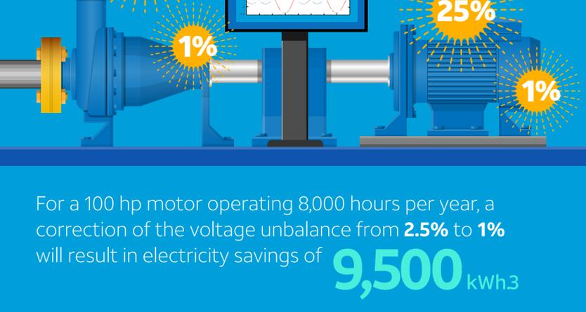
For a 100 hp motor operating 8,000 hours per year, a correction of the voltage unbalance from **2.5%** to **1%** will result in electricity savings of **9,500 kWh<sub>3</sub>**
