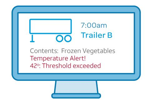
Trailer temperatures are continuously recorded. Alerts are triggered automatically when specified limits are exceeded so the company can take appropriate action.
