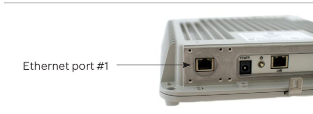
Figure 8 - Ethernet cable connection point
